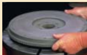
2. Lay the flywheel on the adapter
